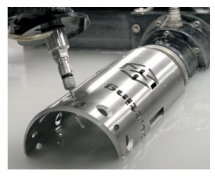
When used with the A-Jet, fishmouth intersections, saddle cuts, and countersunk holes can be cut along the circumference of pipes.
